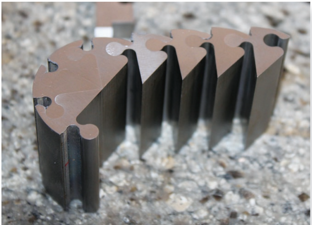
Webster Test Cut Showing Surface Finish and Fit
